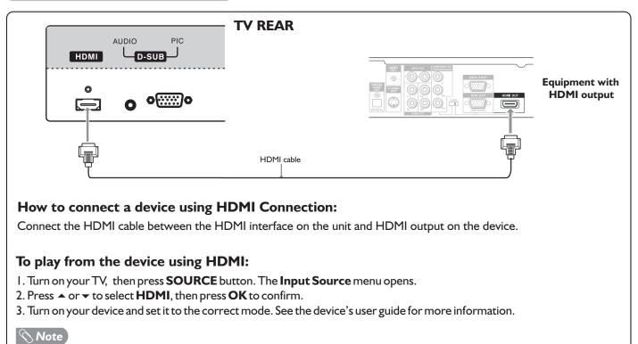
If the external device has DVI output only, use a DVI to HDMI adapter cable to connect to the HDMI terminal. Connect the audio cable to the D-SUB AUDIO IN jack on the TV rear.
